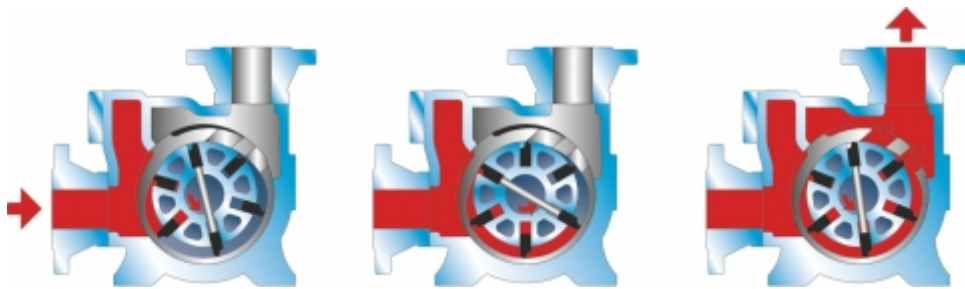
Working Principle of Petroland PV Series Pumps
